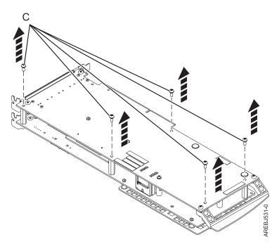
Figure 24. Location of screws on the 572F/575C card set adapter
