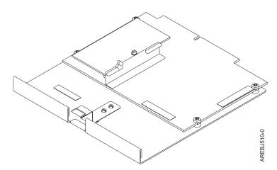
Figure 3. CCIN 57B8 planar RAID enablement card
