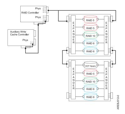
Figure 16. Example RAID and AWC controller configuration
