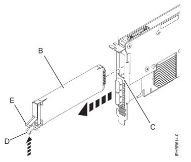
Figure 21. Replacing the 574E cache battery
