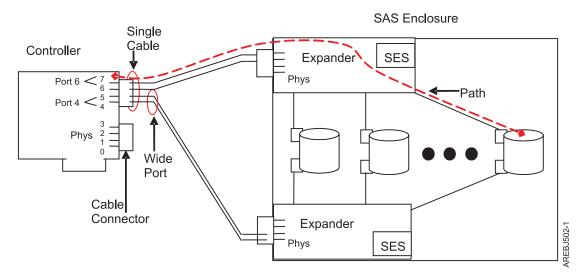
Figure 10. Example SAS Subsystem
