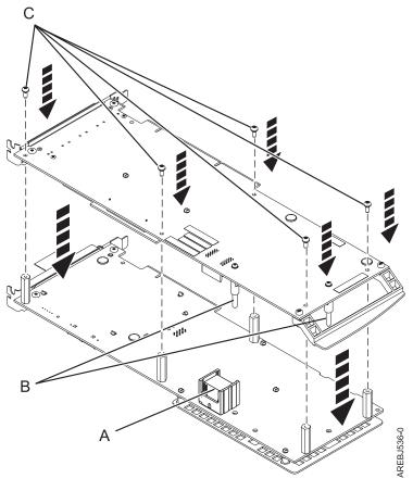
Figure 28. Reassembling the cards
