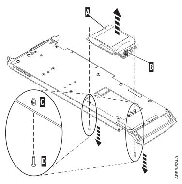
Figure 18. Removing the cache battery
