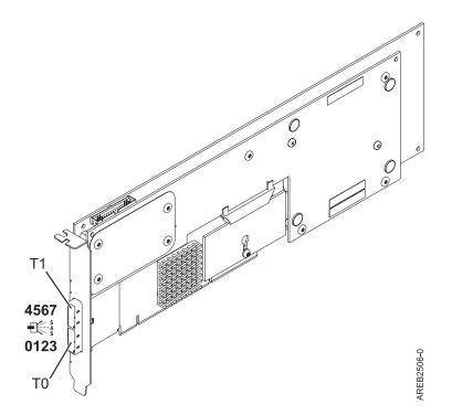
Figure 2. CCIN 572B PCI-X266 Ext Dual-x4 3 Gb SAS RAID adapter
