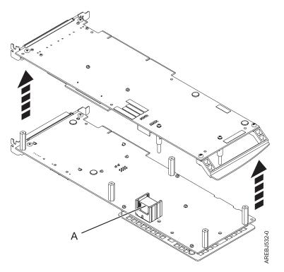
Figure 25. Location of interconnect connector on the 572F/575C card set adapter
