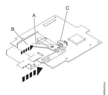
Figure 20. Replacing the 57B7 cache battery
