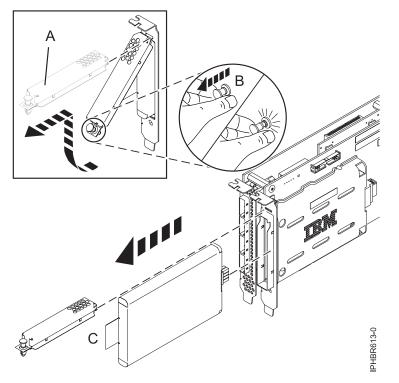
Figure 22. Replacing the 572F/575C cache battery
