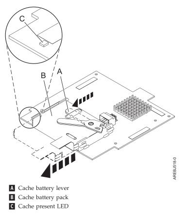
Figure 19. Removing the 57B7 cache battery
